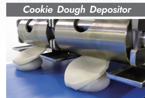
Round "pasta" is deposited and positioned on the dough ball.
