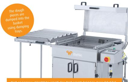
THE MANUAL CONTROL UNIT ON THE LINIE 2000M CAN BE PRO-GRAMMED FOR THREE FRY PROGRAMS WITH UP TO FOUR TURNS; THE DISPLAY SHOWS REMAINING FRY-TIME, AND AN ACOUSTIC TURN AND FRY-TIME END SIGNAL IN CONJUNCTION WITH THE TURNING BASKET ENSURES PRECISION DEEP FAT FRYING
